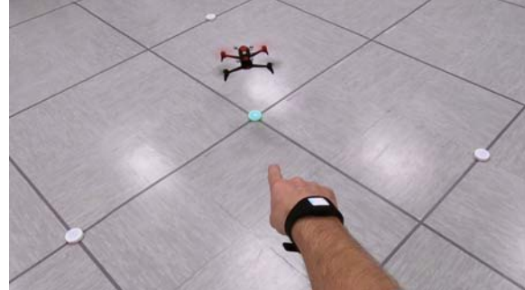
Fig. 1. First person view of the operator equipped with a wrist-mounted IMU interacting with a quadrotor.
