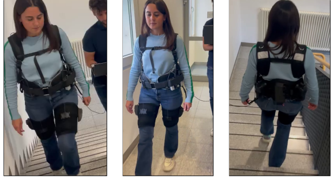
Fig. 1. We equip an easy-to-wear and light exosuit with a user-tailored perception model estimating the current and intended walking gait (ascending or descending stairs and walking on level ground) using only IMU readings.
